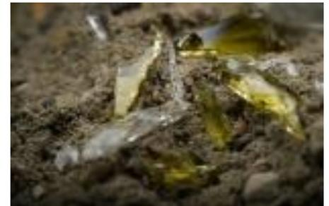
*MSU researchers have found that concrete is more durable when crushed glass is added to the cement used to make the concrete. Photo by G.L. Kohuth*
