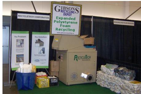
Gibsons Recycling use "thermal densification" equipment to recycle Expanded Polystyrene Foam (EPS)
